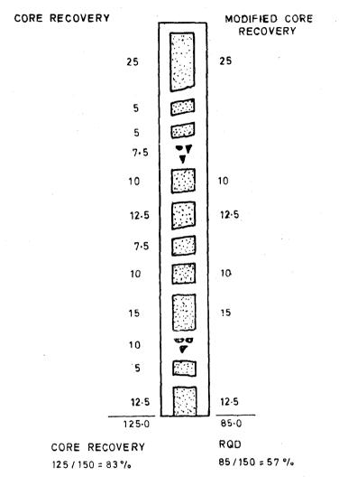
FIG. 1 MODIFIED CORE RECOVERY AS AN INDEX OF ROCK QUALITY.
